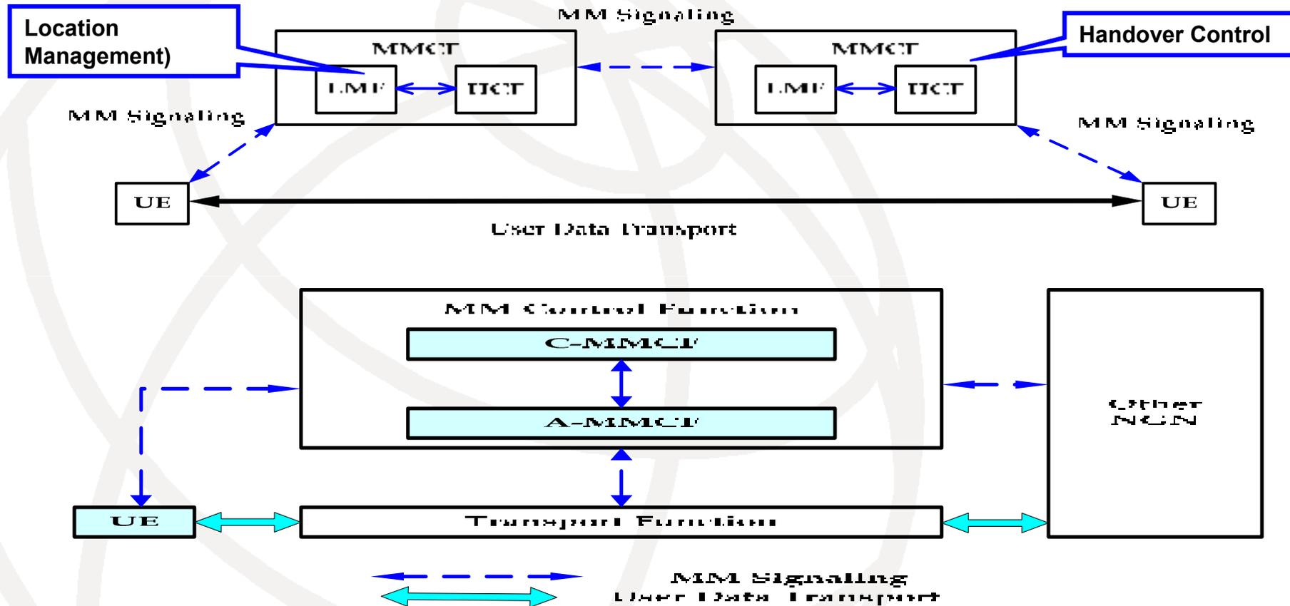
Functional architecture-level view of Mobility Management Control Function (MMCF) in NGN [Y.2804/Q.1707] - MMCF is located in NGN Transport Control
